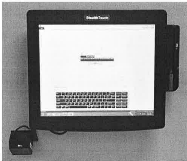
A PTS kiosk at a room entrance to scan in and out a volume via its individual barcode.
